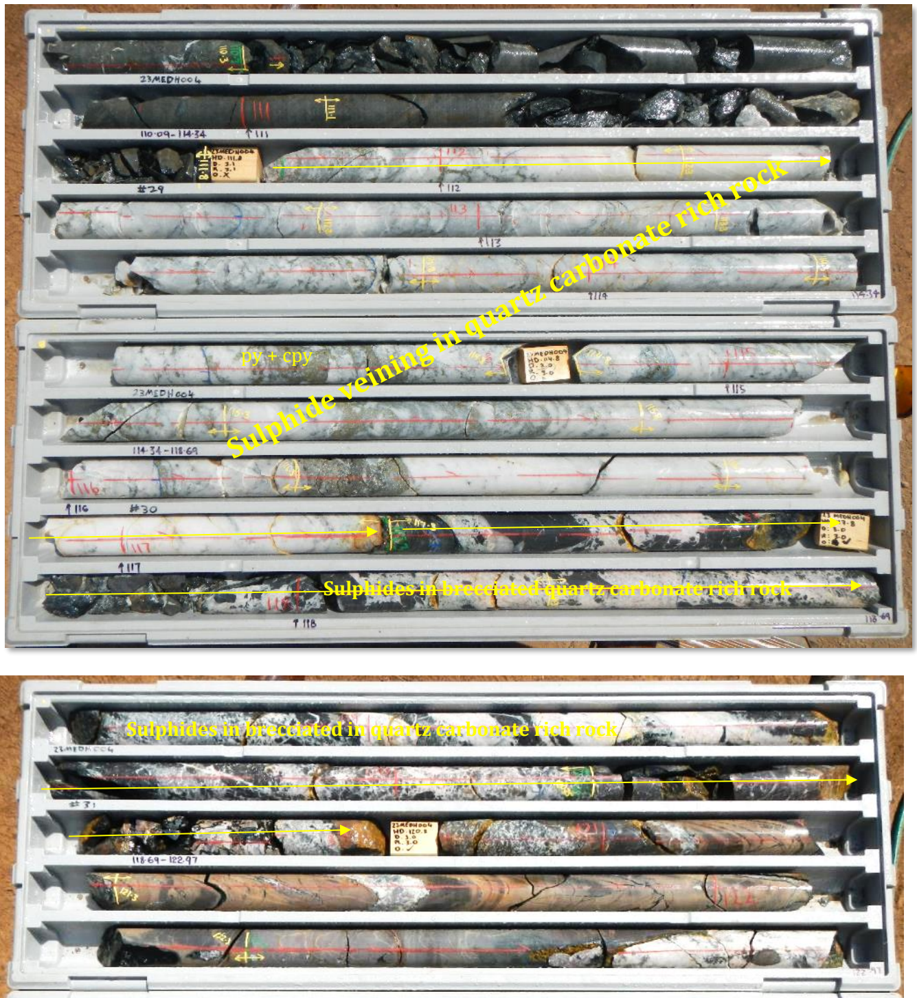
Plate 3: core from drill hole 23MEDH004 (~111m to 121m) showing sulphide mineralisation
