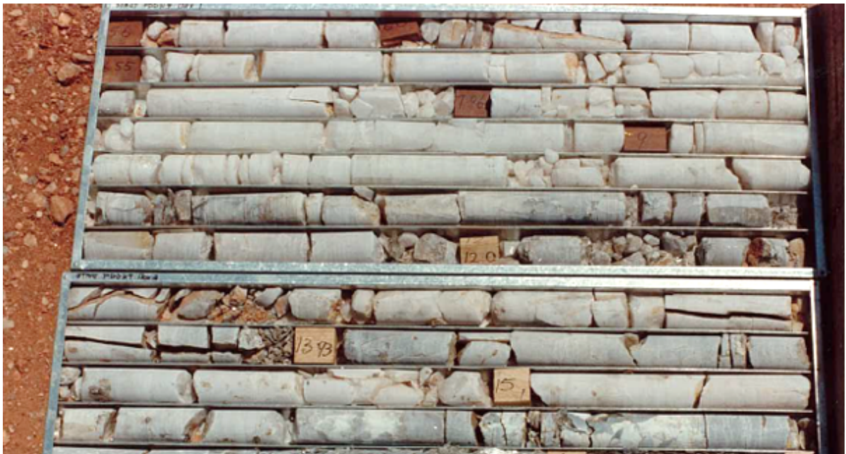
Plate 3: Historical drill core for hole PDDH9. Massive quartz from 5.6m to 15.5m. (Wamex Report A33097)
