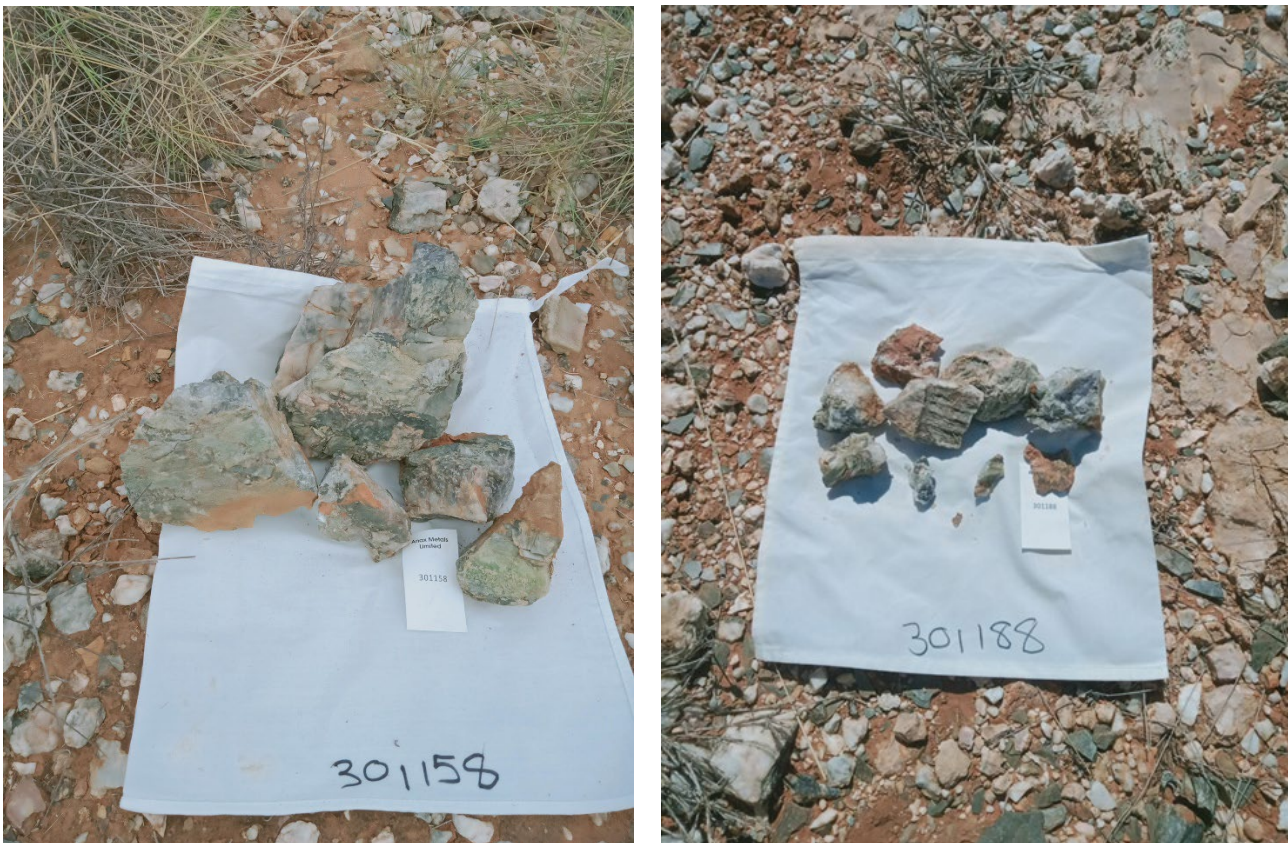
Figure 3: Lithium bearing minerals in pegmatite samples from Whim Maar Prospect. (301158 -potential green coloured spodumene minerals. Li =20ppm; 301188 - relict spodumene textures evident. Li =38ppm) 7,9
