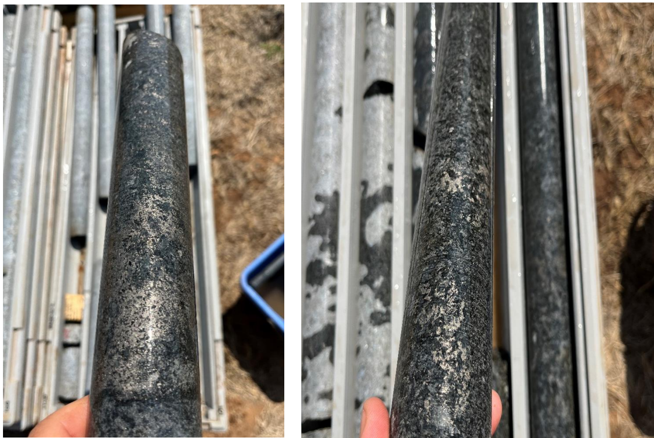
Figure 1. Photos showing examples disseminated and blebby sulphides in hole BRDD002. (Left) Nickel-Copper sulphides at 348m, (Right) Disseminated sulphides 338 – 342m Note core is NQ2 being 2 inches or 50mm in diameter
