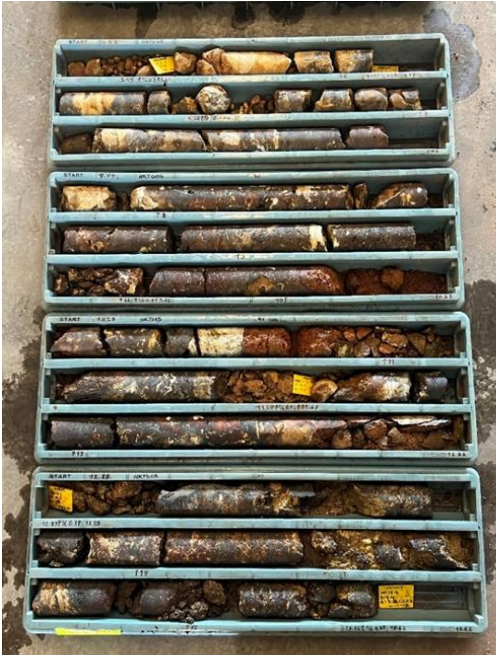
Appendix 3. Hendeka PQ3 diamond core samples from hole HKT005 (trays 2-5 photographed below) were included in master composite HKT002-005.
