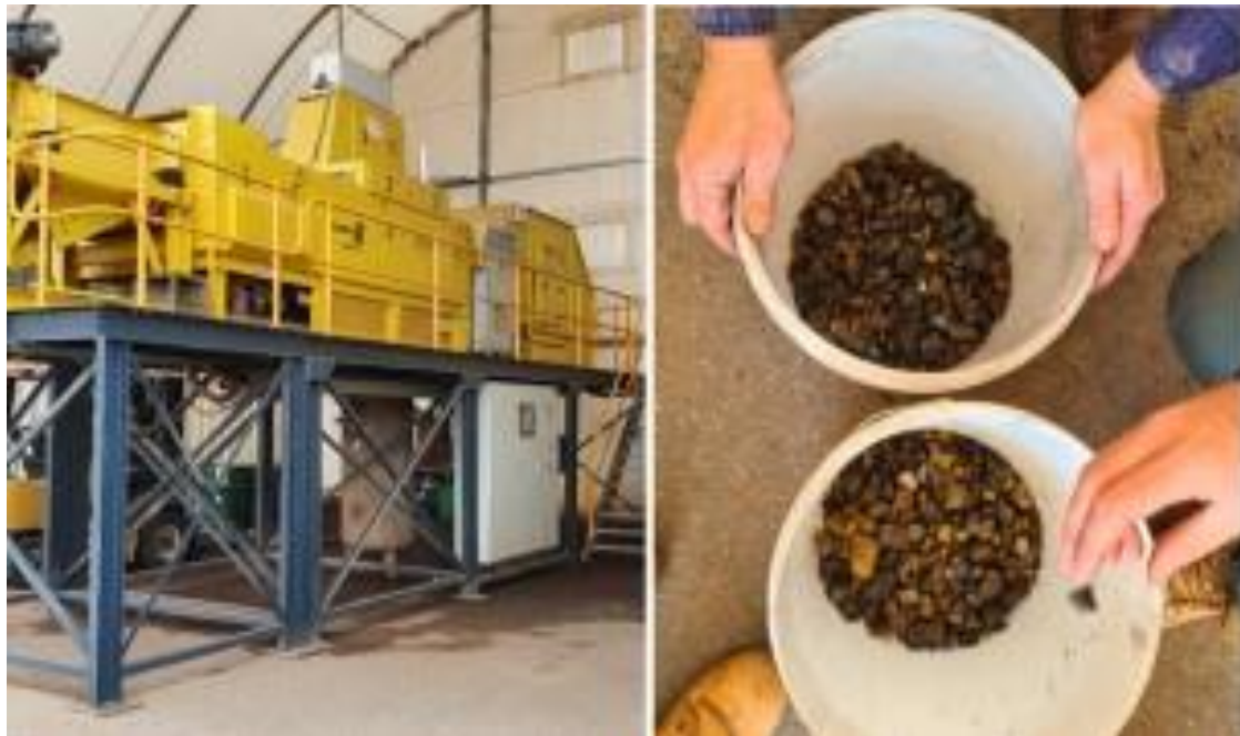
Figure 3. The Steinert ore sorter at Bibra Lake, Perth that was used to test +10mm samples from Hendeka (LHS) and the resultant material with Product top and Waste below (RHS).
