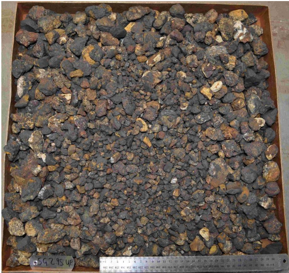
Figure 2: +6.3mm Ericsson Cone Concentrate
