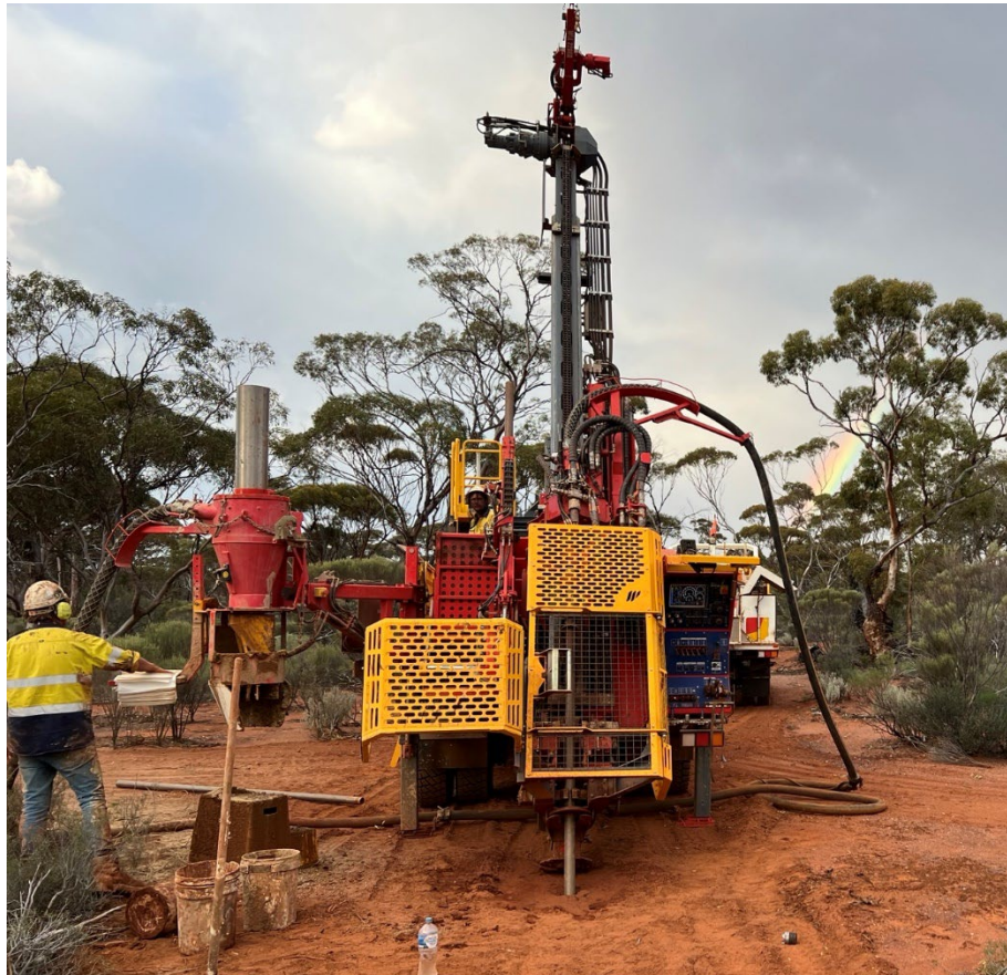
Figure 1: Aircore drilling completed at Ryans Find.
