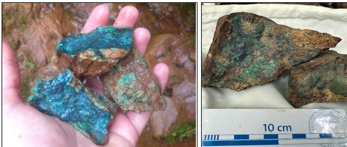
Figure 4 - Sample REG-104923: 20% Cu and 1540ppm – displaying massive chalcocite, azurite and malachite (LHS) and ST008: 6.5% Cu and 155ppm Ag displaying malachite and azurite in sandstone.
