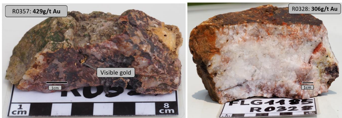
Figure 1a: Visible gold identified in quartz vein samples at Salane (LHS) and high-grades in white quartz (RHS).
