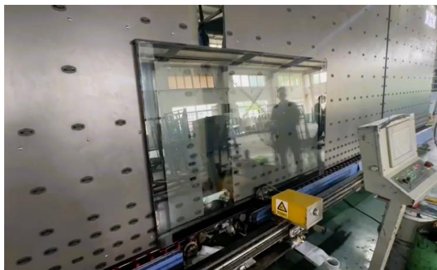
ClearVuePV vision glass IGU being manufactured on a standard IGU production line.
