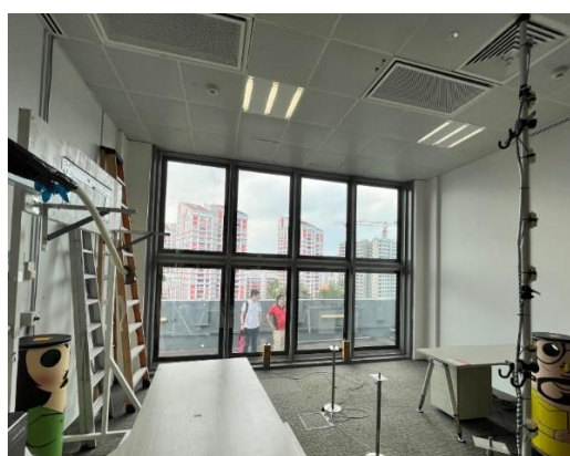
Second Generation ClearVuePV vision glass testing IGU's and spandrel panel units (above the glazing) installed and being prepared for commencement of BCA testing.
