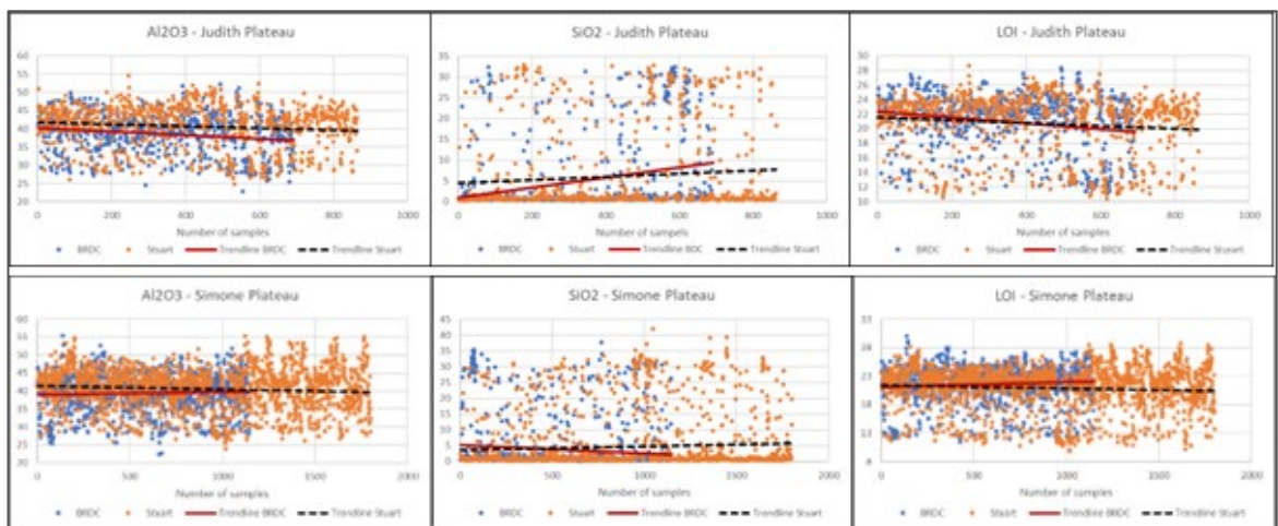
Figure 6.1: Comparison of BRDC and Stewart laboratory databases (2009) for Judith and Simone plateaus
