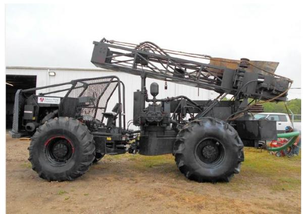
Figure 2: Soil test borehole drilling rig.
