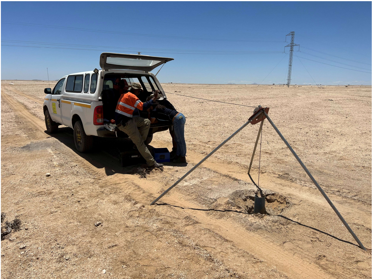
Figure 4 Downhole Gamma Probing at Koppies 3
