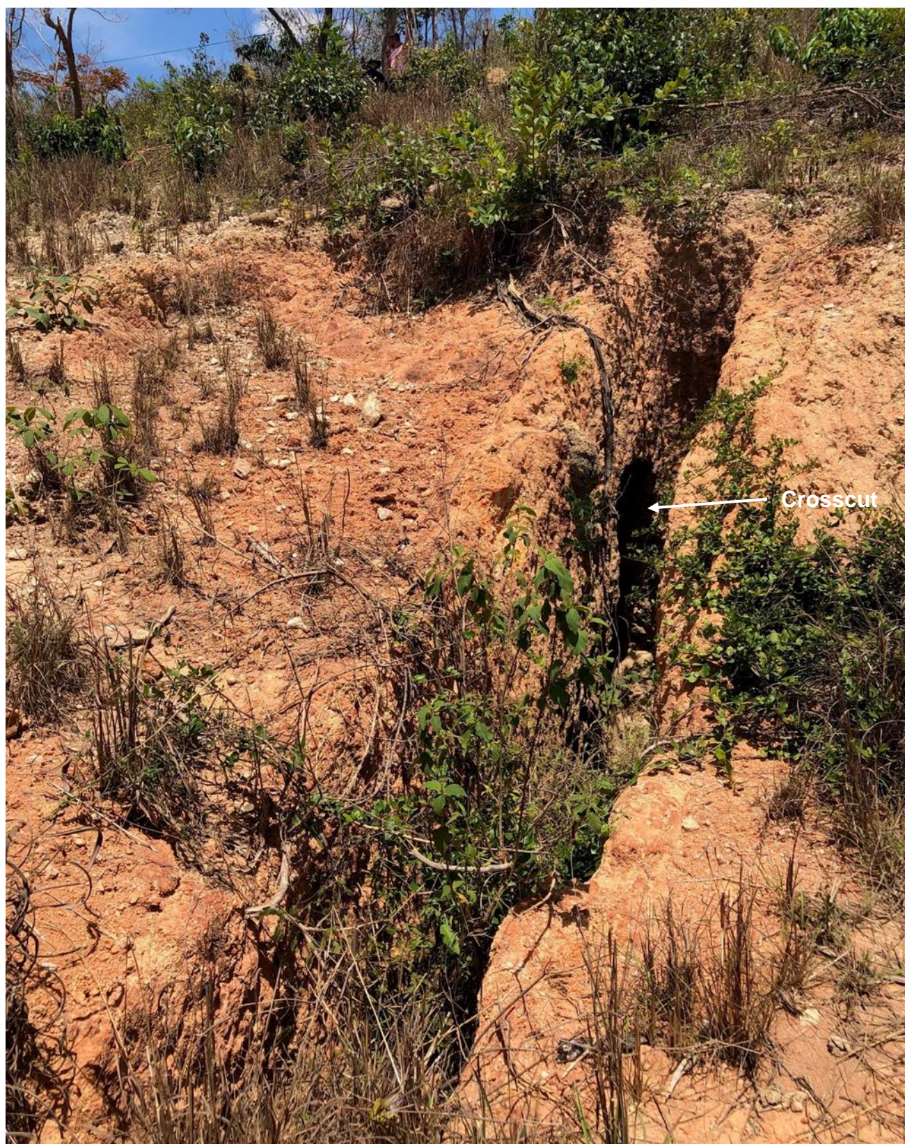
Figure 4: Carai artisanal mine workings for emeralds and green tourmaline. The workings consist of a 7m x 1m trench with crosscuts either side. There are also a number of shallow pits on the uphill side of the trench.
