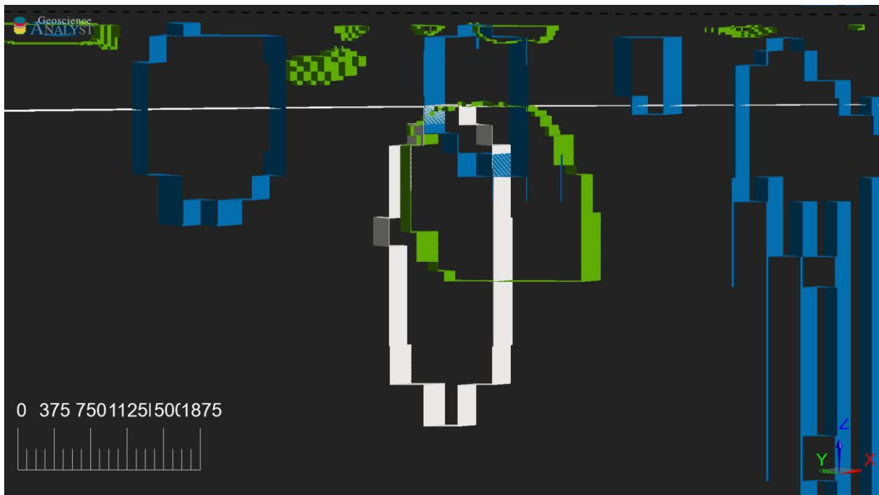
Figure 4: Section view of the Parker 3D interpretation model — looking northeast at density, magnetic susceptibility, and conductivity iso-surfaces from Table 1. Magnetic susceptibility ( -0.0025 SI) is cloud white, ZTEM conductivity ( 0.002 S/m) is earth green, and density is sea blue ( -0.023 g/cc). The horizontal white profile is the interpreted unconformity surface (Bosman et al., 2020).
