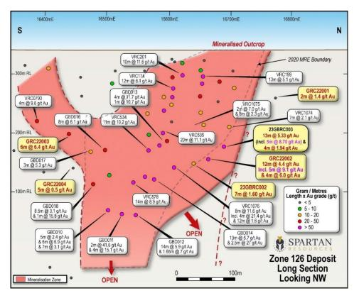
Figure 5: Long Section of the Zone 126 Gold Deposit showing both historic and recent assays (yellow). Recent assays include 13m @ 5.33g/t gold (23GBRC003) and 12m @ 4.4g/t gold (GRC22002)
