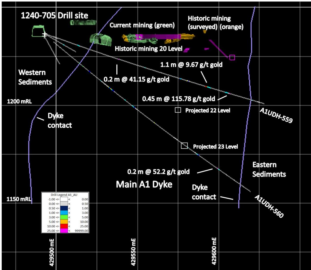
Figure 5: Cross section viewed north along 120 Mine grid azimuth, illustrates the location of the drillholes A1UDH-559 and - A1UDH-560 drilled from the 1240-705 drill site, with respect to the A1 Mine workings, reported in this announcement. Modern drives (green) and the interpreted historic workings (magenta) and modern surveyed (orange).
