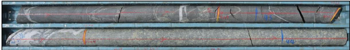
Figure 1: 0.2m @ 9.0 g/t gold from 43.23m at the contact with the western sediments and dyke, between 21-22 Levels.
