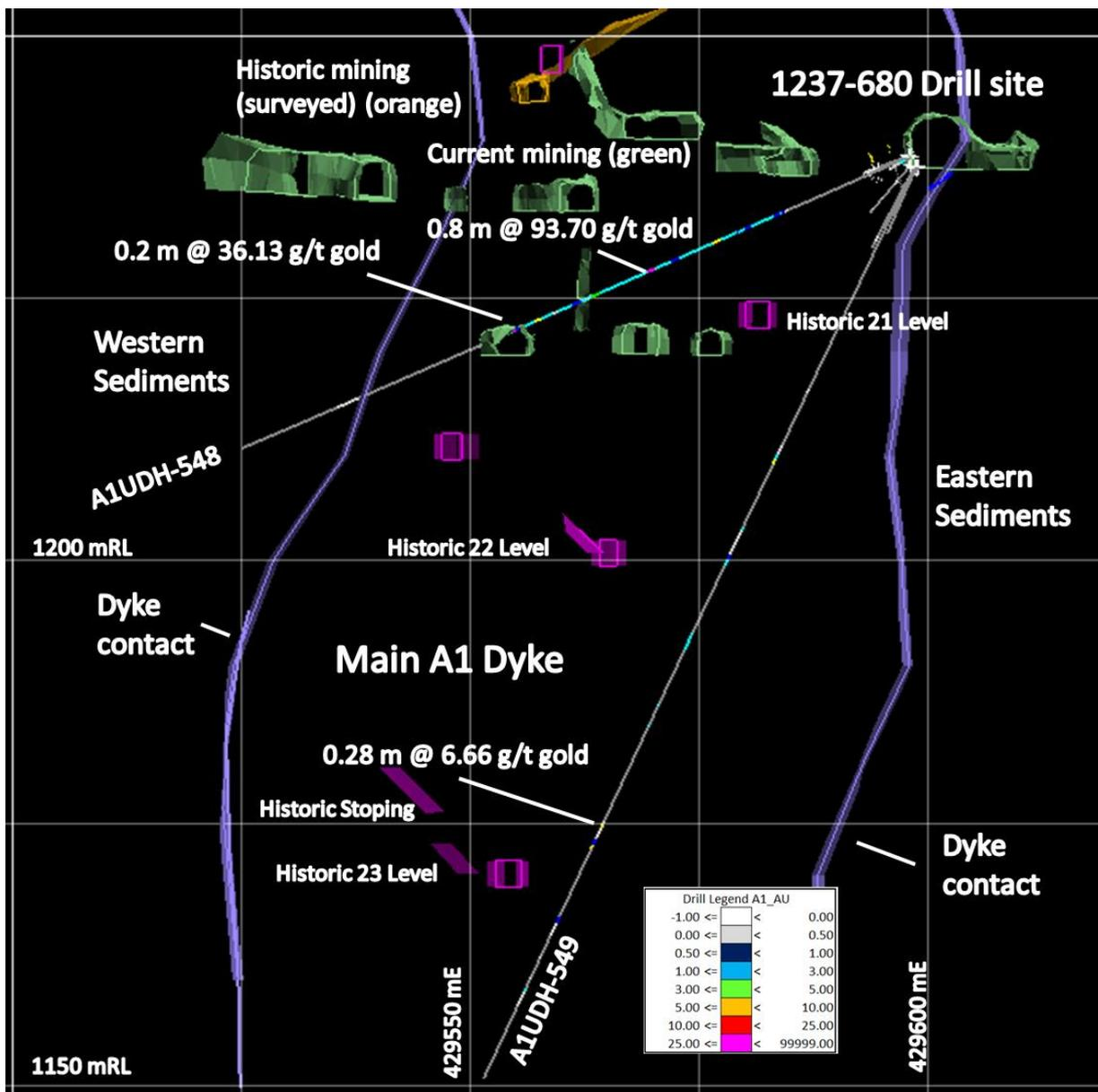
Figure 4: Cross section viewed north along 240° Mine grid azimuth, illustrates the location of the drillholes A1UDH-548 and - A1UDH-549 drilled from the 1237-680 drill site, with respect to the A1 Mine workings, reported in this announcement. Modern drives (green) and the interpreted historic workings (magenta) and modern surveyed (orange).
