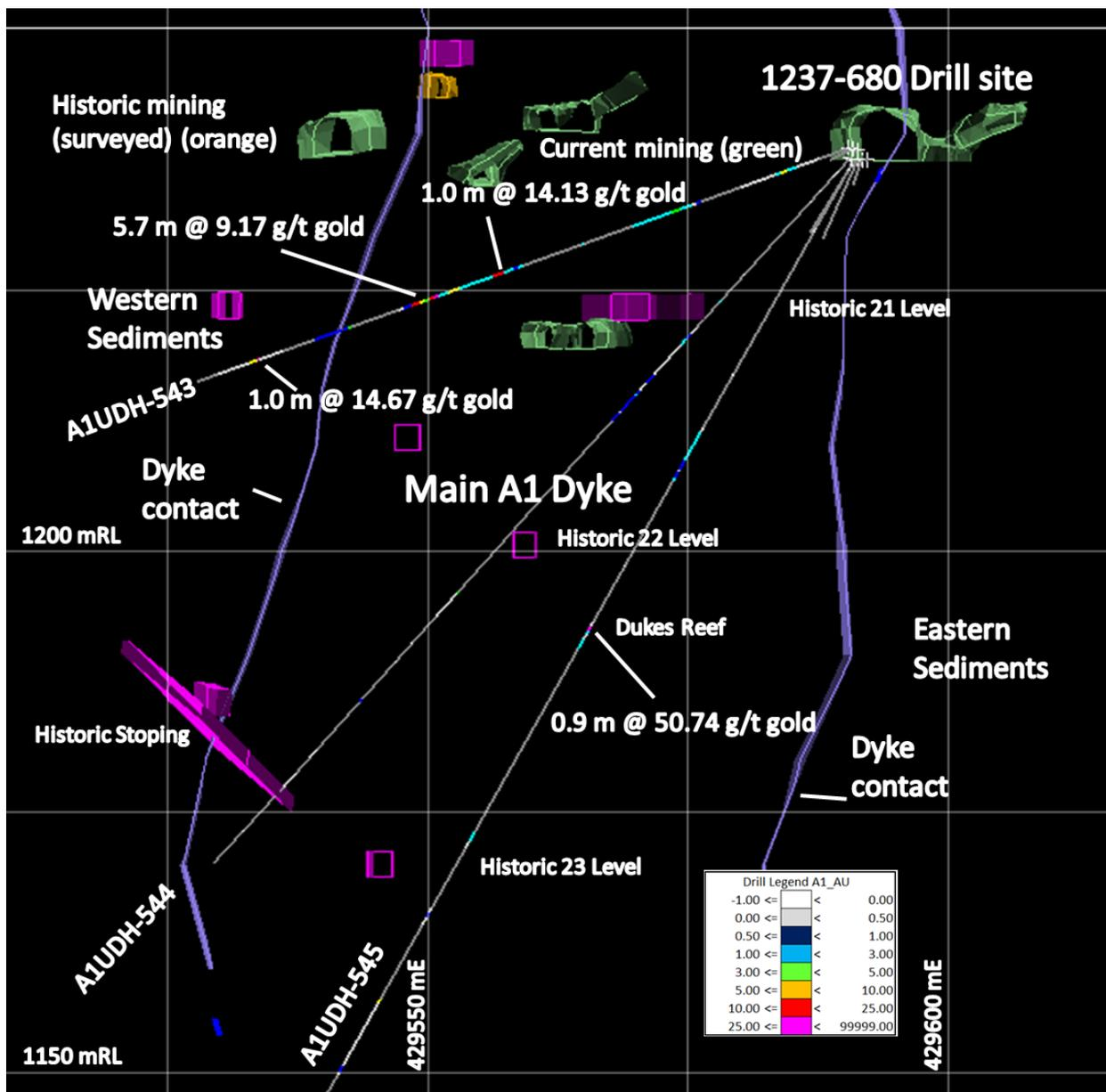
Figure 3: Cross section viewed north along 260° Mine grid azimuth, illustrates the location of the drillholes A1UDH-543, -544 and -545 drilled from the 1237-680 drill site, with respect to the A1 Mine workings, reported in this announcement. Modern drives (green) and the interpreted historic workings (magenta) and modern surveyed (orange).
