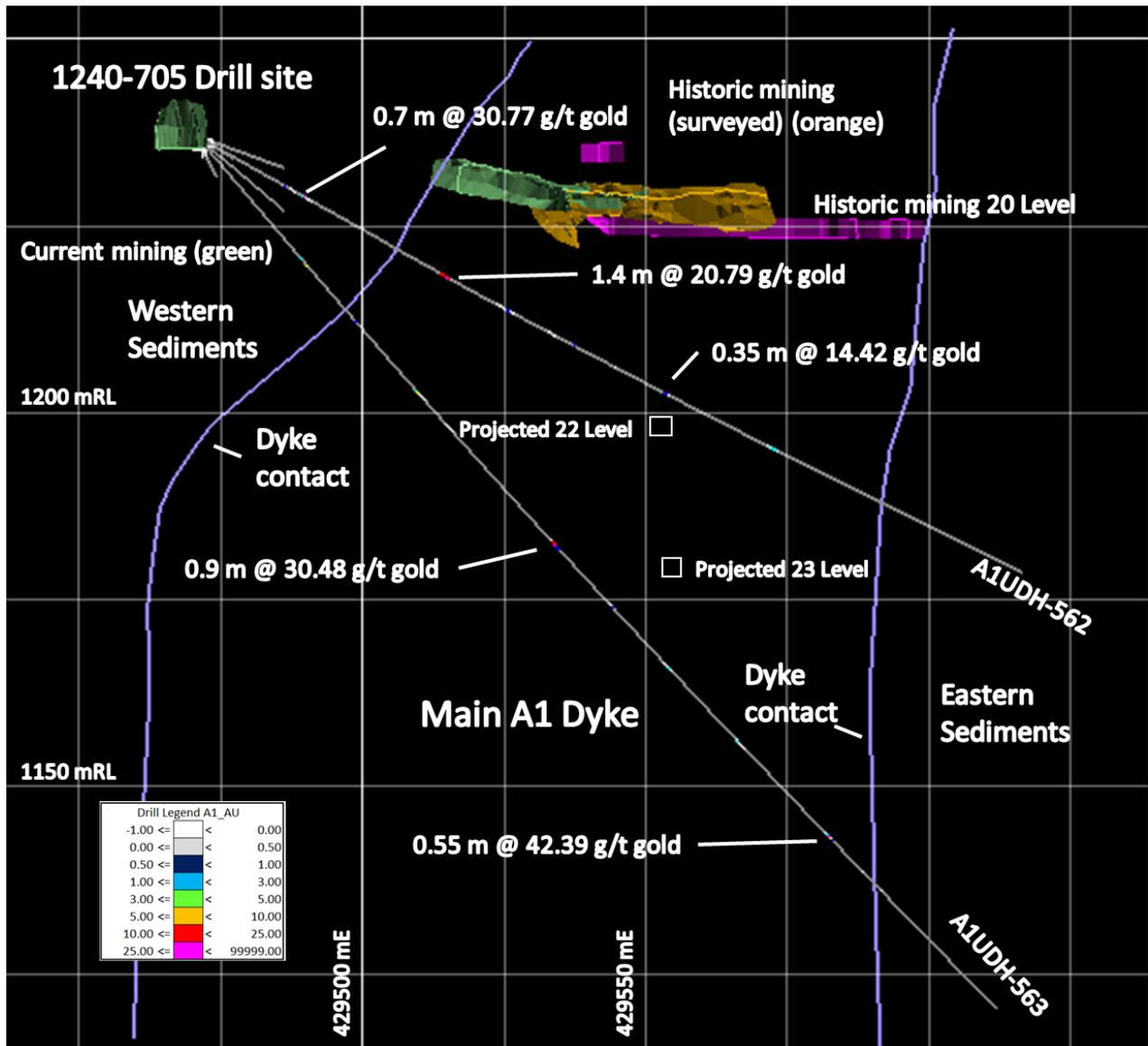
Figure 6: Cross section viewed north along 130 Mine grid azimuth, illustrates the location of the drillholes A1UDH-562 and - A1UDH-563 drilled from the 1240-705 drill site, with respect to the A1 Mine workings, reported in this announcement. Modern drives (green) and the interpreted historic workings (magenta) and modern surveyed (orange).
