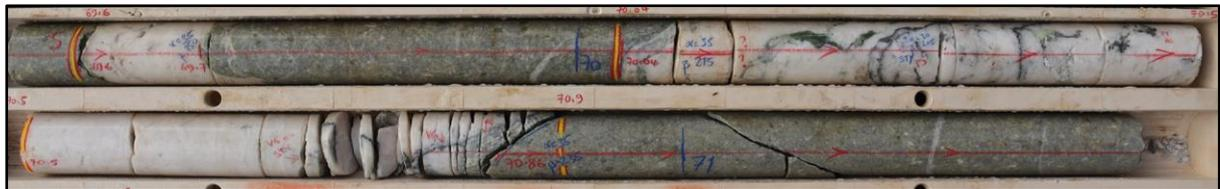
Figure 2: 0.9m @ 30.5 g/t from 70m with significantly mineralised stylolitic sulphides and many specks of visible gold along some of these. This lies between 22-23 Levels.
