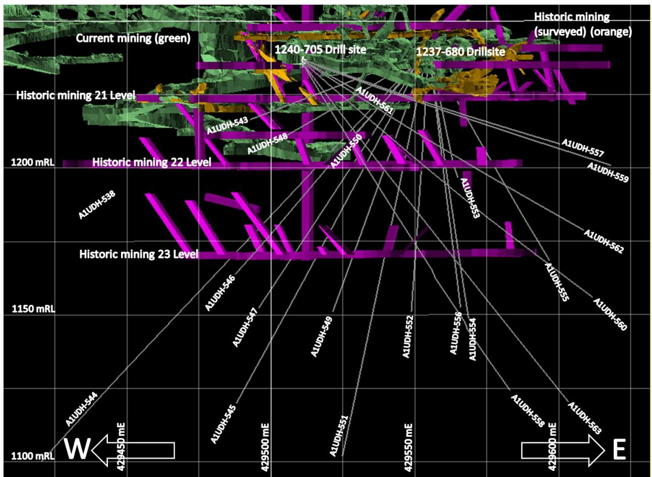
Figure 7: Oblique section viewing north showing drilling traces (grey), modern drives (green) and the interpreted historic workings (magenta) with some recent survey pick-ups (orange).
