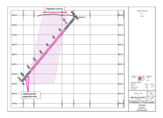
Figure 2: Cross section showing the pegmatite intersection of BDFS02
