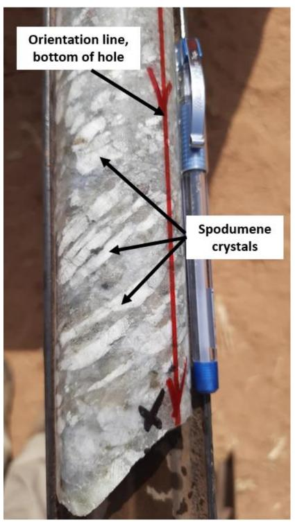
Figure 3: Spodumene in drillhole BDFS02
