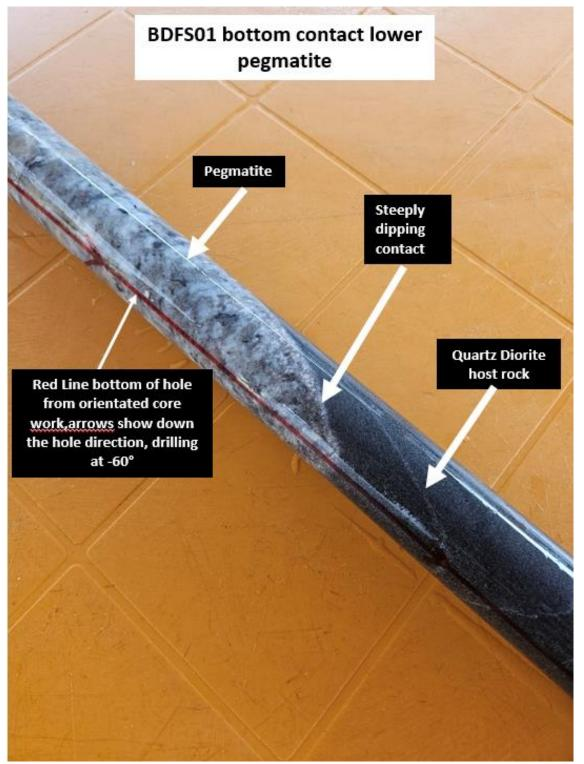
Figure 4: Bottom contact of pegmatite in BDFS01 showing the steeply dipping contact
