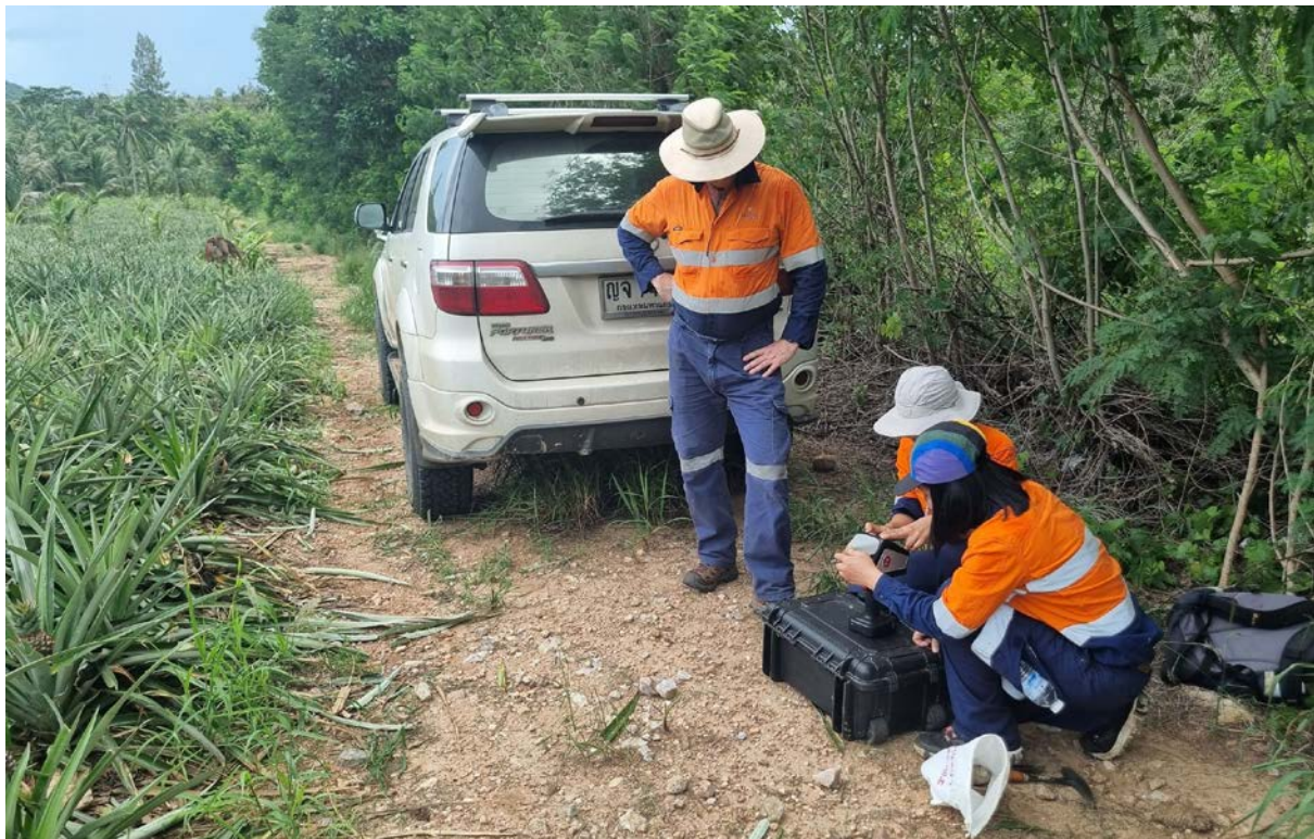
Photo 3: Matsa director, Pascal Blampain with the Matsa Thai geological staff undertaking field assessment of rock sample using SCIAPPS LIBS (laser induced breakdown spectroscopy)
