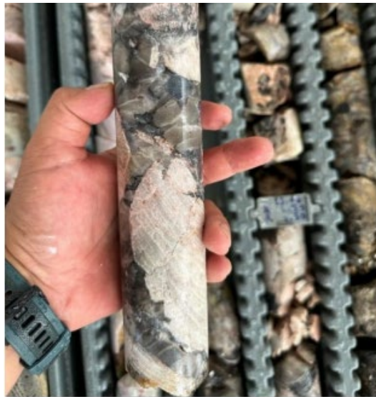
Figure 5: Coarse spodumene crystals in JADDH0002 (34.05m) within weathered brecciated quartz rich core of the Jaguar pegmatite
