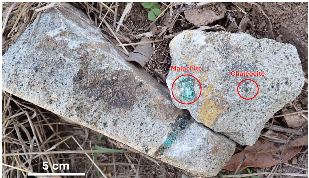
Figure 9. Specimen sample from the field of sub-porphyrific andesite, containing malachite and chalcocite blebs, from Kaa prospect.
