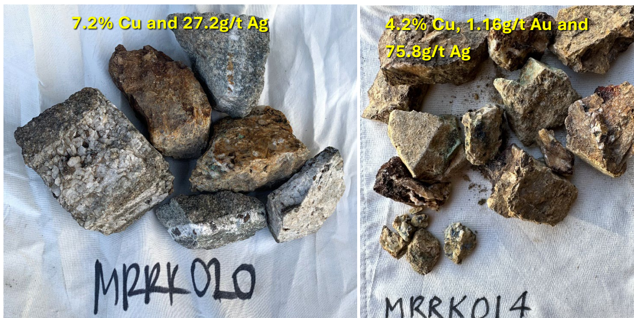
Figure 2. Rock chip sample MRRK020, bornite crystals, 1 cm x 0.5cm in size, within quartz veins, at the contact between a mafic and a granite unit. MRRK014, iron rich quartz vein at surface.
