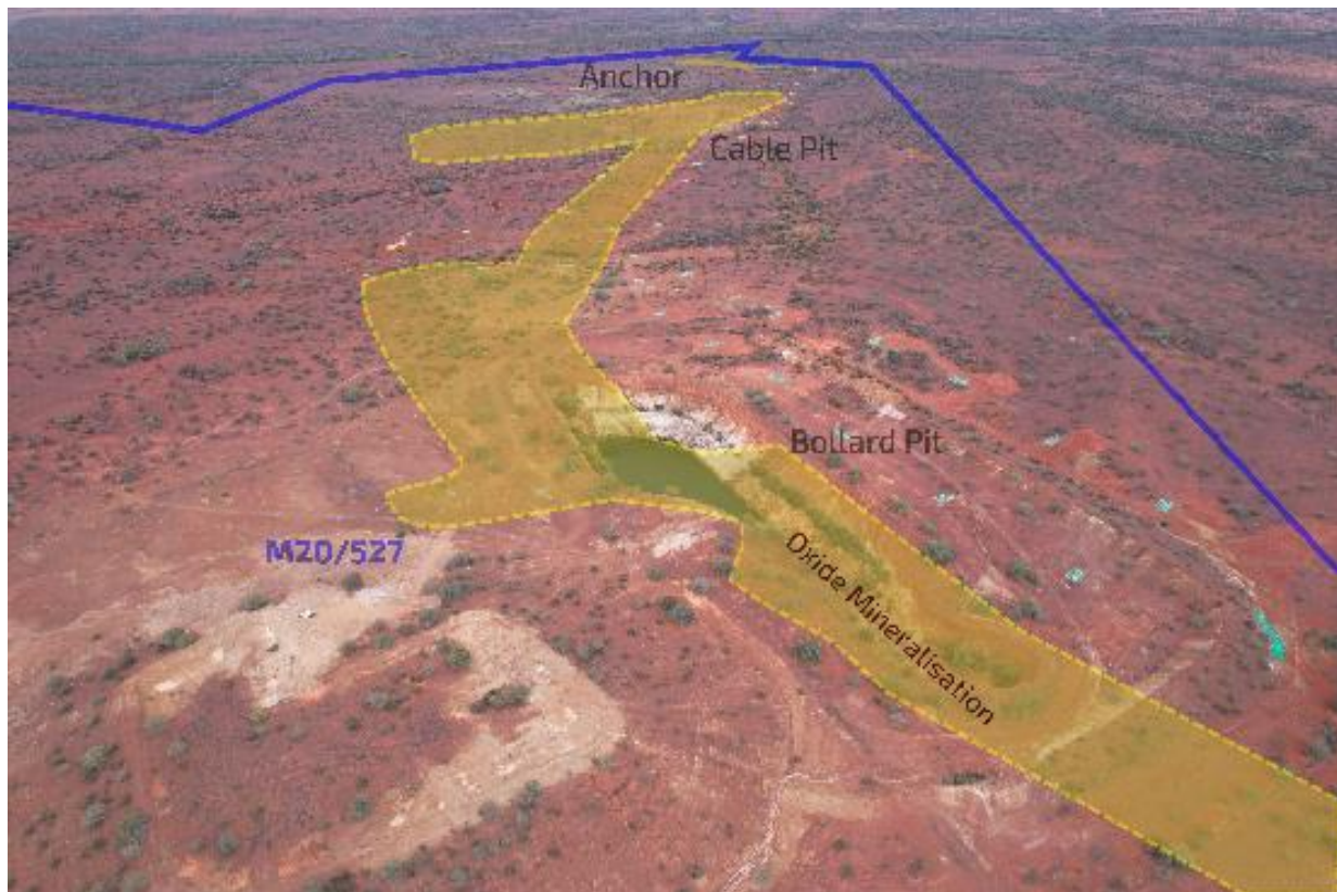
Figure 2: Shallow oxide gold mineralisation (yellow) on the granted mining lease (blue outline) extends for over 1.7km of strike.
