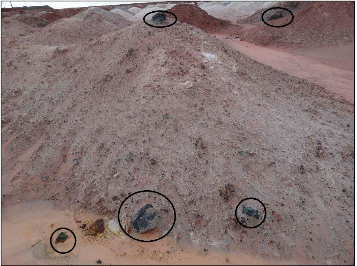
Image 5: Pimple dump on CIP tailings cell- part of composite sample (7,193,821mN 663,814mE) – DSO material circled.
