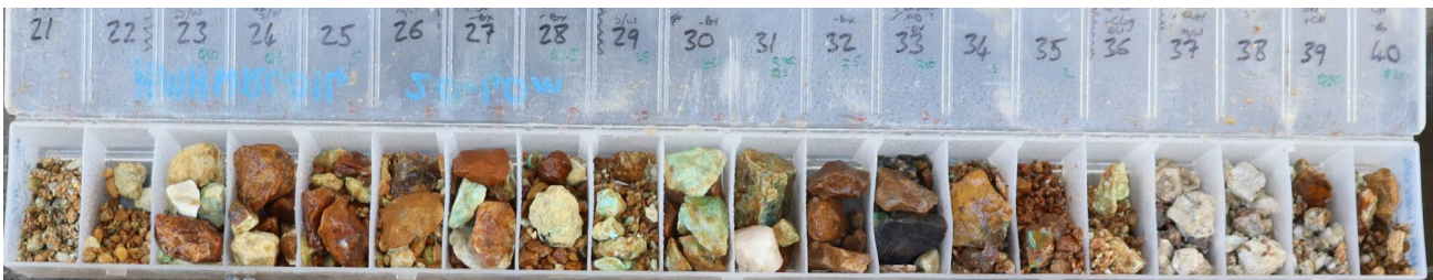
Figure 2. Copper oxide visible in drill chips from HMHWRC0014 (20-40m). A copper grade of 2.78% was reported between 31m and 36m (See Table 1).
