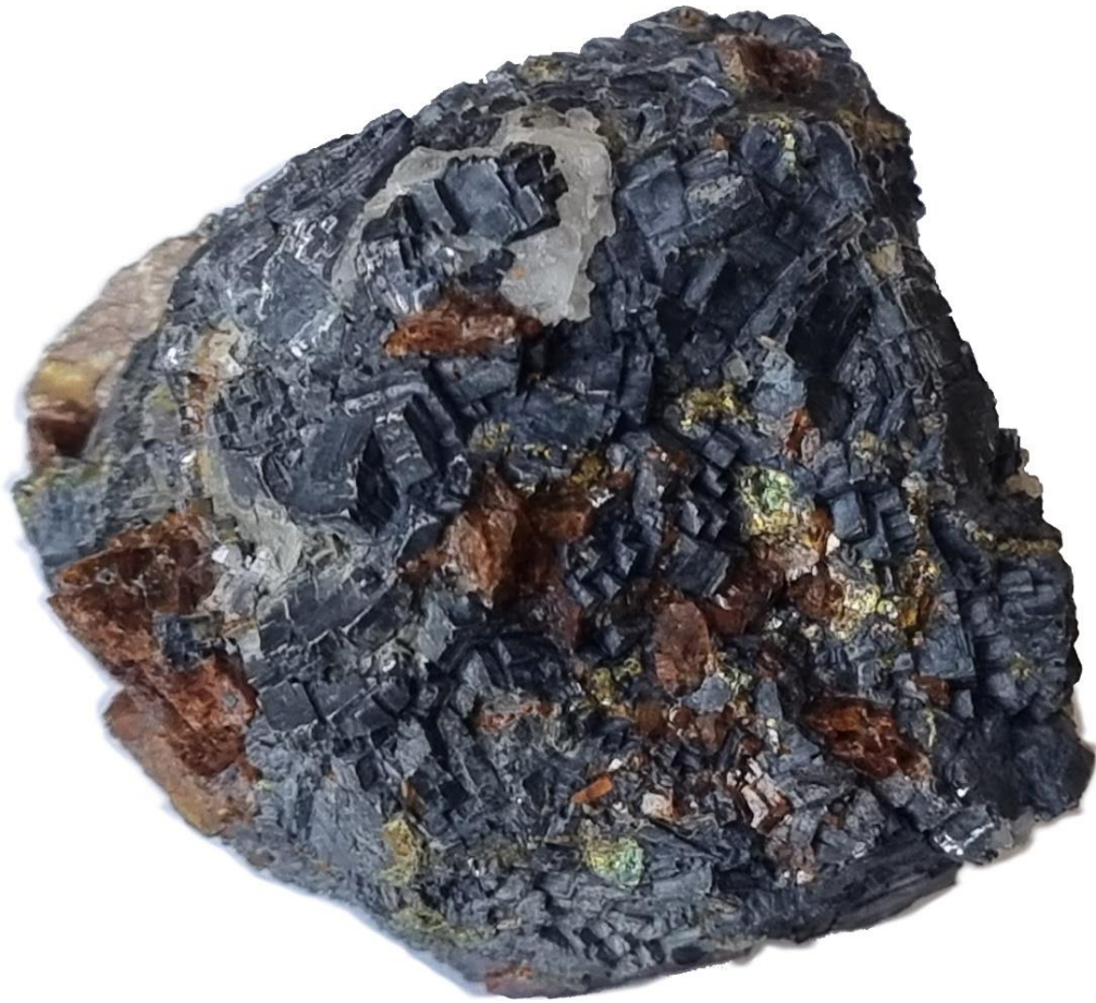
Figure 102: Mineralised waste dump specimen visually estimated to consist of 70% Galena; 10% Chalcopyrite; 10% Sphalerite and 10% Quartz
