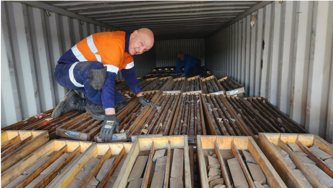
Image 2 - View of inside of sea container – with the drill cores stored in 3m long trays.
