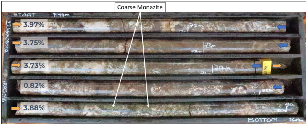
Image 1: Carbonatite with green coarse monazite mineralisation visible. KGKDD002 71.44m to 76.09m
