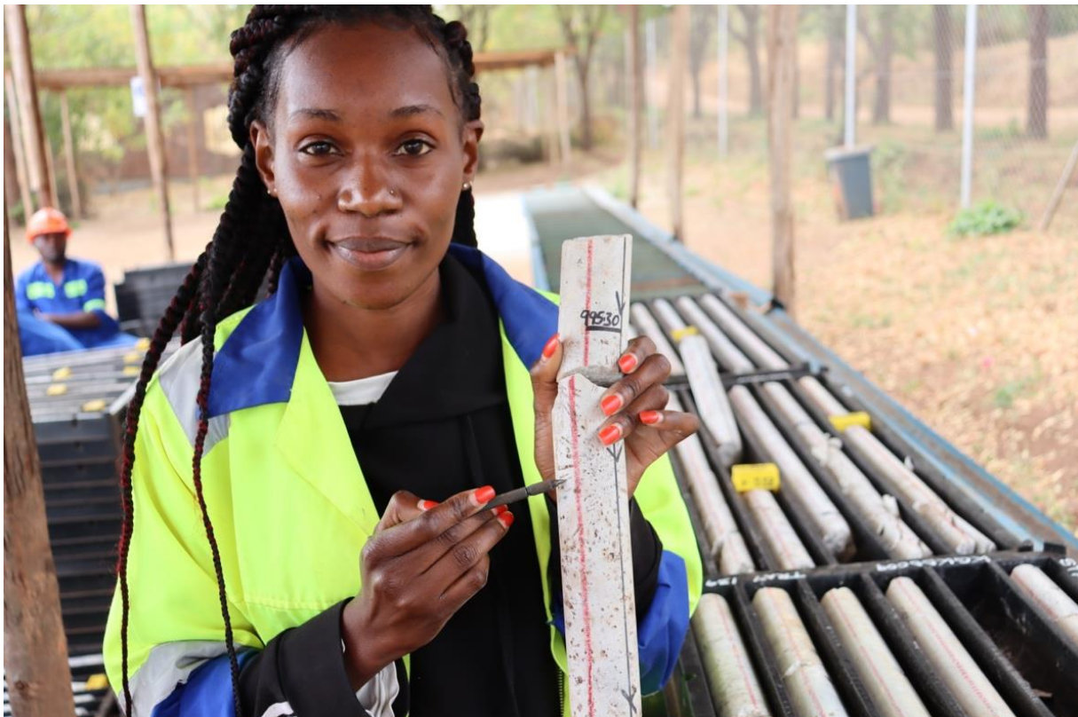
Image 4: Serah Misuku, Site Program Geologist, with a section of drill core showing textural features of monazite, strontianite and baryte (replacing original burbankite crystal pseudomorphs) at 995.3m downhole. Intersection 995.30 to 995.72 for 0.42 metres at 7.09% TREO. Refer ASX announcement of 18 September 2023 titled "SECOND DEEP DRILL HOLE INTERCEPTS 1,000 METRES OF MINERALISATION GRADING 2.6% TREO"
