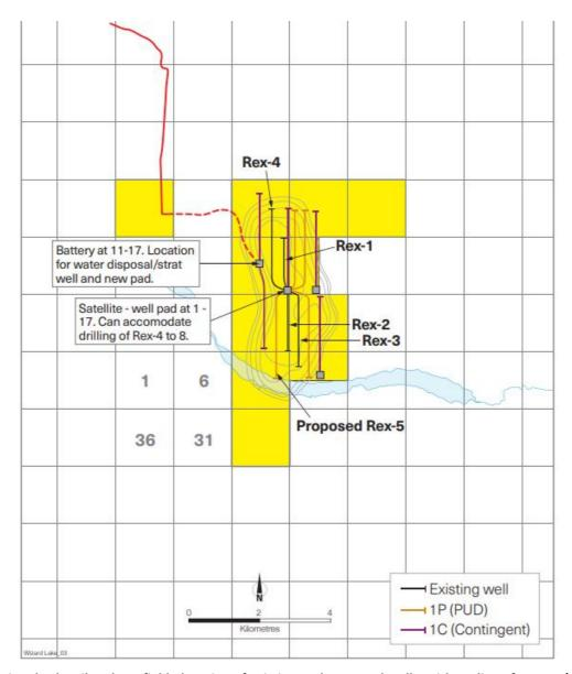
Figure 1 – Wizard Lake oil and gas field - location of existing and proposed wells, with outline of Proven (1P) reservoir
