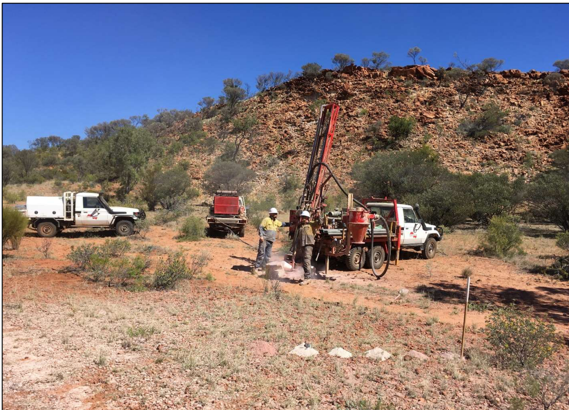
Figure 4 – Aircore drilling at the Dingos Rest South prospect August 2023.
