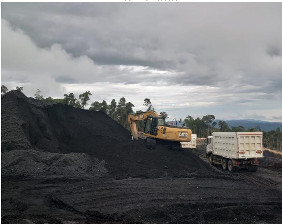
Coal loading at ROM stockpile BBM Pit-3
