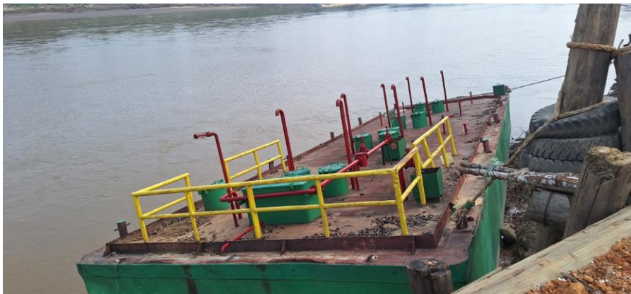
Fuel barge of 400KL capacity is ready to use – at Jetty Batu Tuhup
