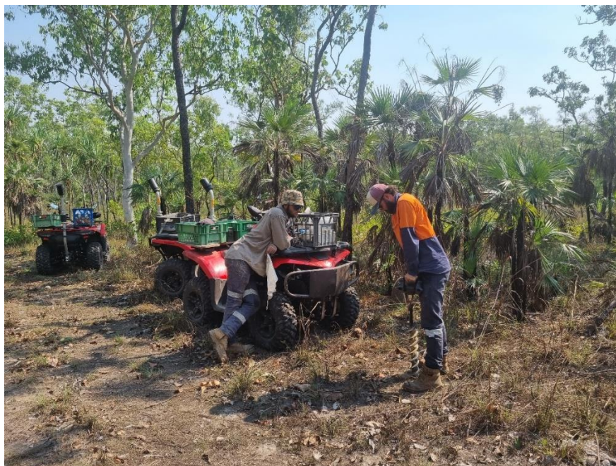
Figure 2: Soil sampling crew taking samples using a hand held auger drill.
