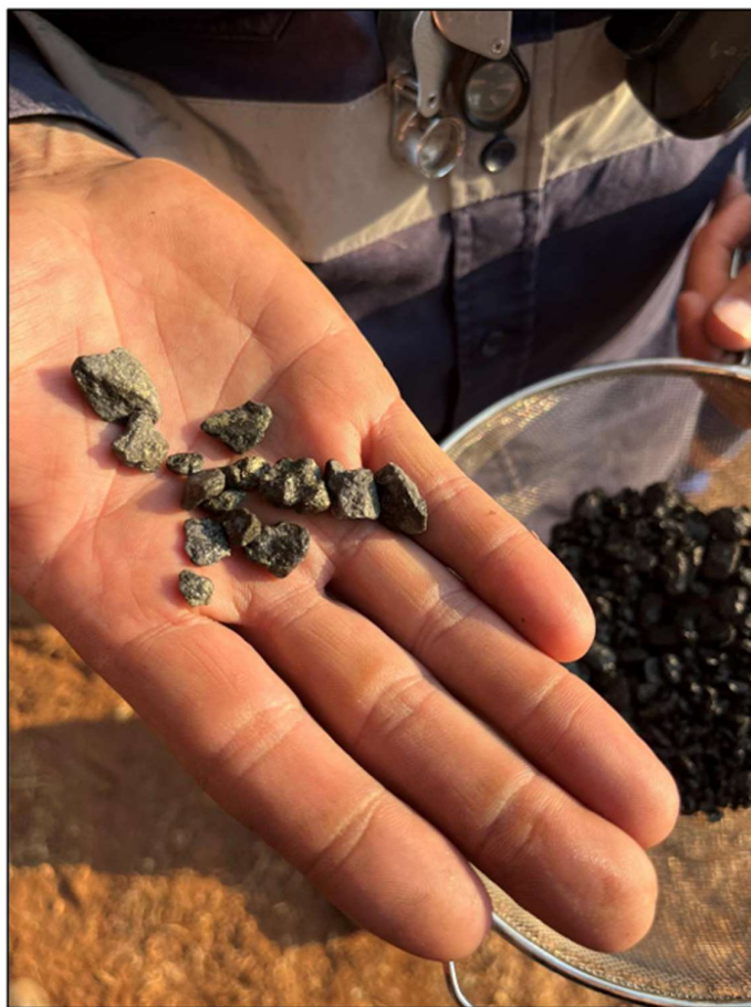
Figure 6: Chalcopyrite mineralisation logged in DBRD141 at 48-49m down hole.
