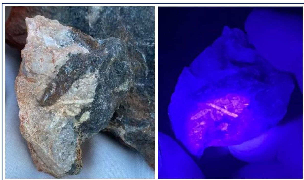
Figure 6. – Hand-specimen of spodumene crystals in LCT pegmatite showing strong pink fluorescence, a characteristic feature under long-wavelength UV light (Sample ID: ESS02321 - Location -28.59985257, longitude 116.8597968).
