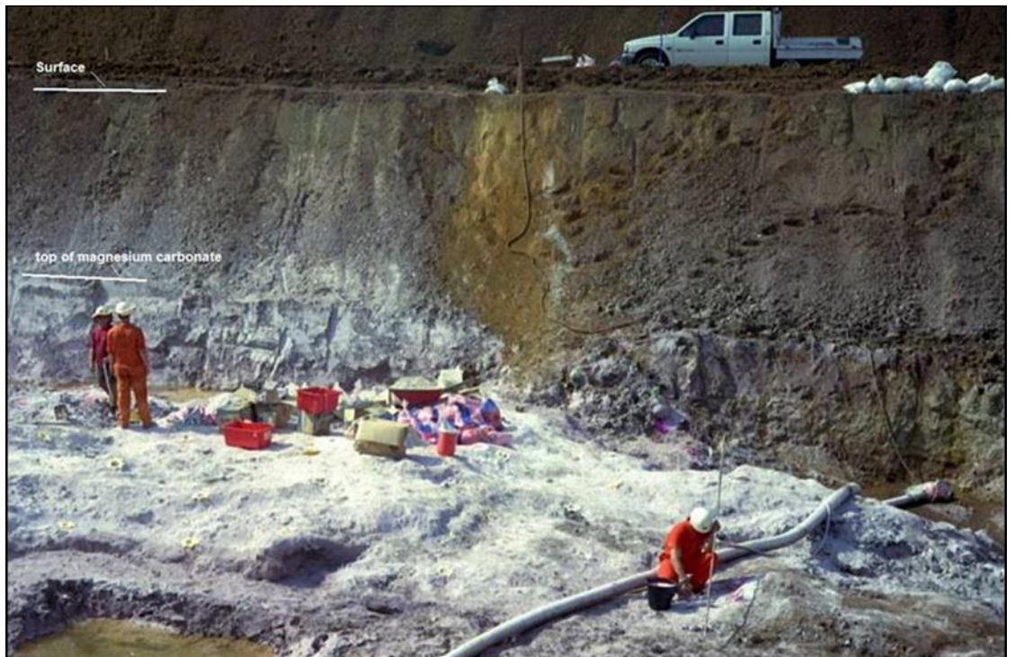
Figure 8 Test mining of magnesium at Winchester during the wet season (preparing to blast Level -1).
