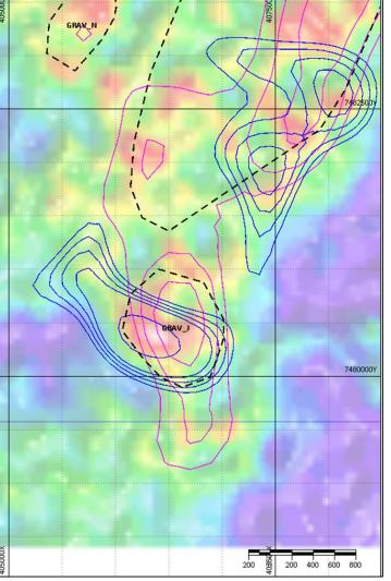
Figure 7: Tantor Magnetic gravity anomalism plan view. Total magnetic intensity (TMI) contours in blue, vertical gravity gradient (GDD) in magenta.
