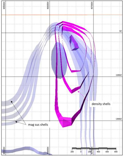
Figure 8: 7480400 cross section. Showing magnetic UBC Model shells in blue and gravity model in magenta
