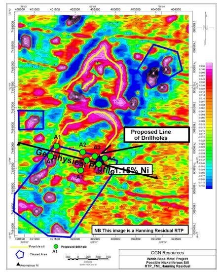
Figure 11: Shep target possible nickeliferous still RTP\_TMI\_Hanning Residual.
