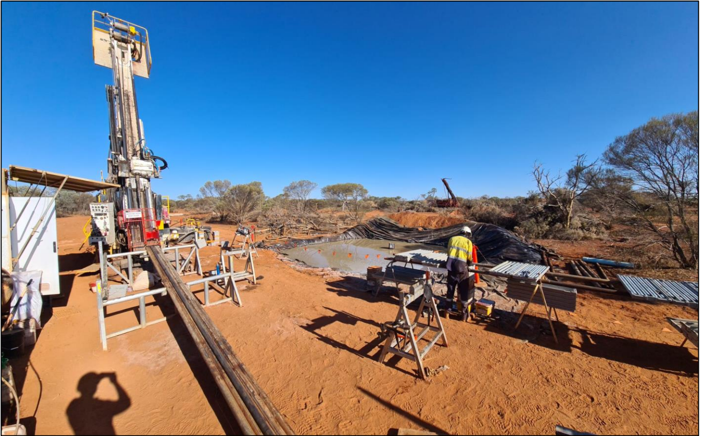
Image 1: Diamond rig completing MWDD001 (foreground) and the RC rig commencing drilling a diamond pre-collar (background)
