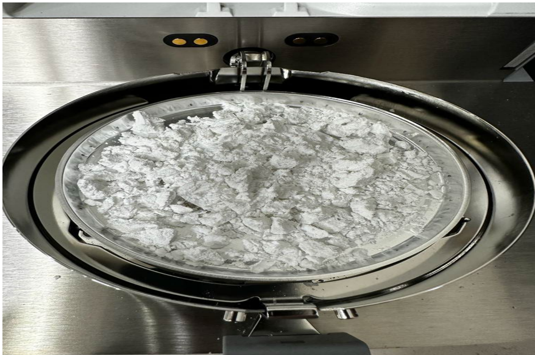
Figure 1- High grade Lithium carbonate produced from Prairie Brine
