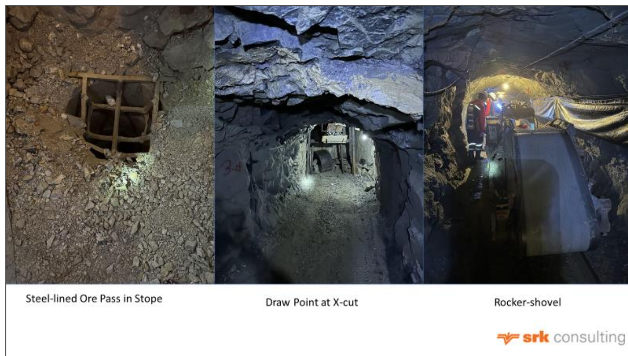
Figure 5-22: Typical underground conditions
