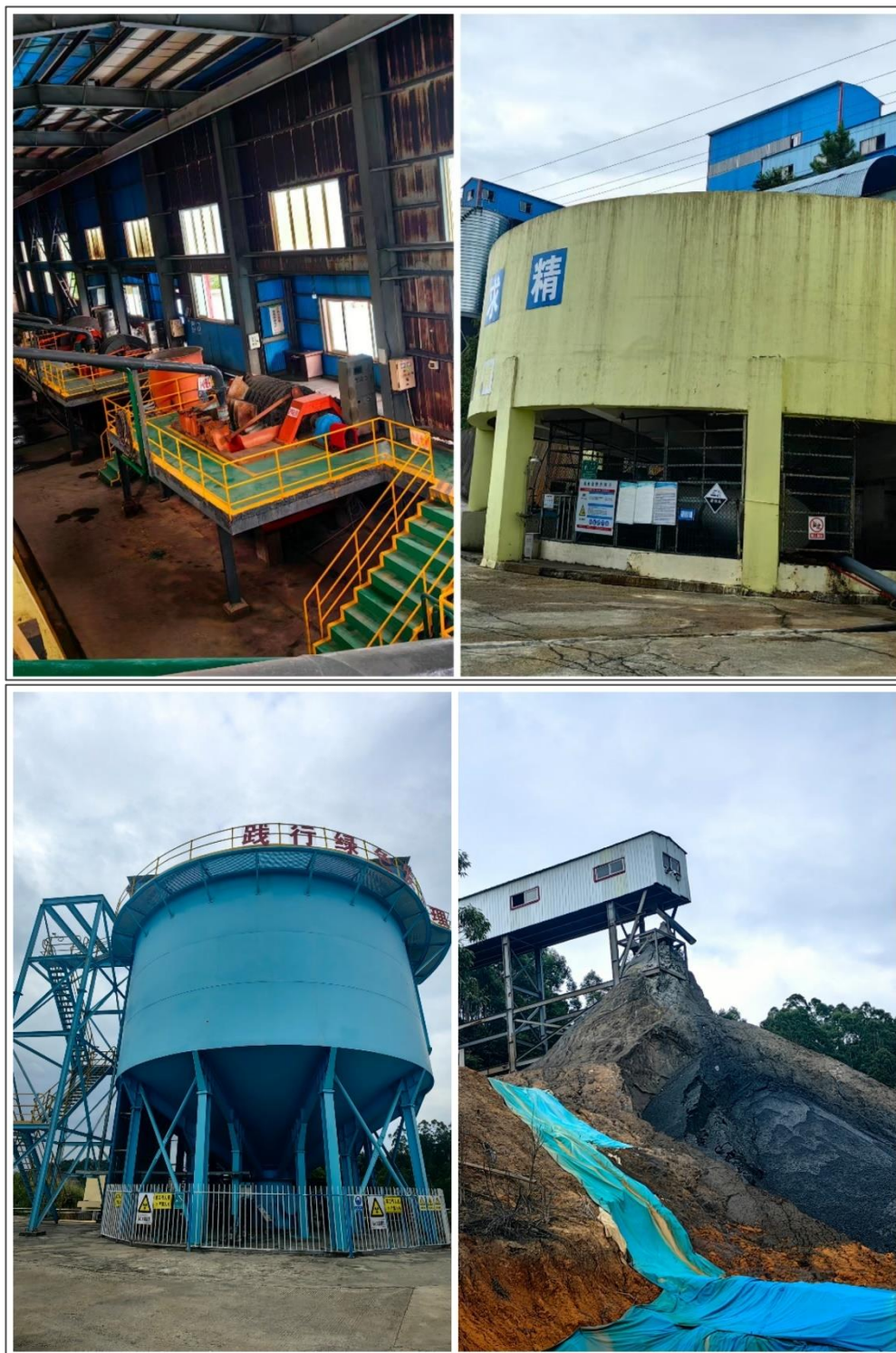
Figure 6-7: Concentrate dewatering and tailings handling
