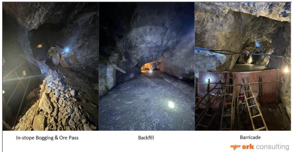
Figure 6-11: Operation of cut and fill stoping
