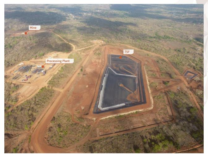
Figure 5: Aerial view from the east of the Project. TSF with the HPDE lining nearing completion in mid-October.
