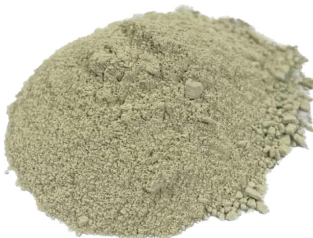
Figure 1. Mixed Rare Earth Carbonate test product produced from North Stanmore
