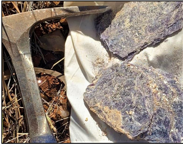
Figure 2: Examples of samples with high lithium and REE assays at QXR's Turner River, Pilbara. (Photo of sample collected in same location as 23QXRX-017 with 3.4% LiO 2 , with 50% mica, 30% feldspar, 20% quartz. See Figure 1 for location)
