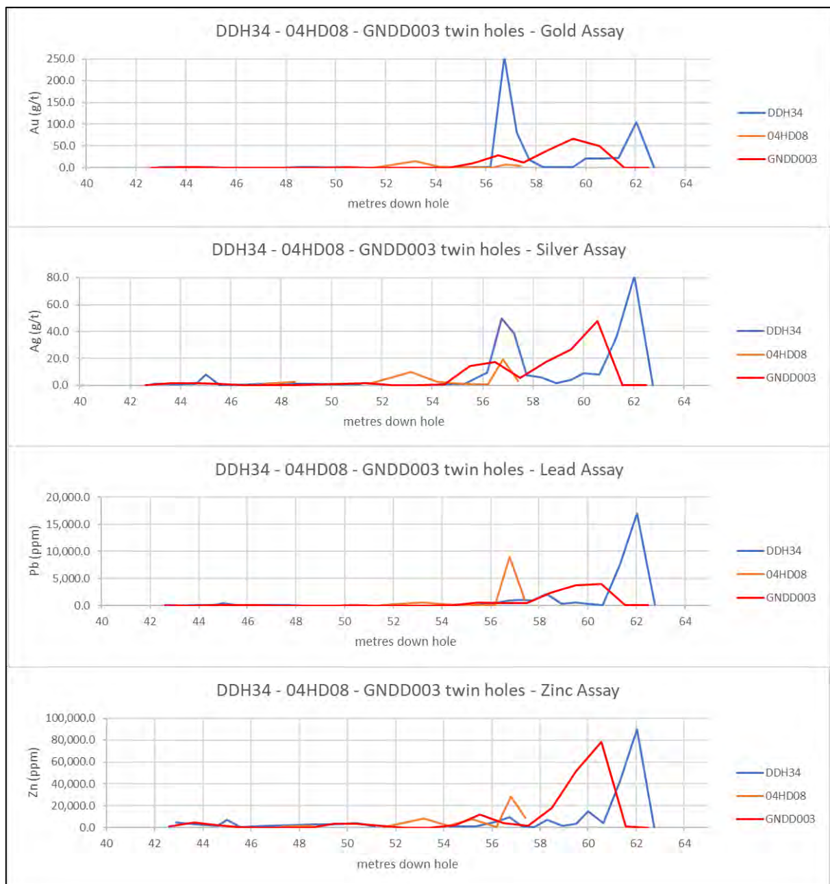
Figure 9-12: Down- hole assay plots for Au, Ag, Pb and Zn from DDH34 and GNDD003 and 04HD08.
