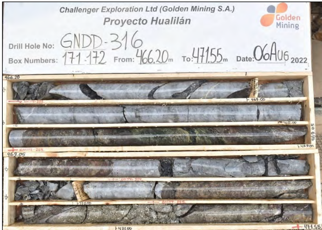
Figure 7-16: Zinc skarn (manto) in limestone (CAL) with overprinting retrograde alteration.
