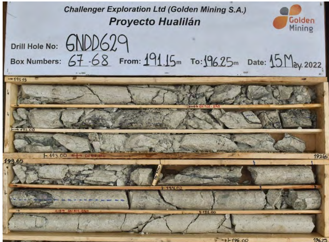
Figure 7-18: Low grade mineralisation formed in narrow veins and disseminated pyrite in altered dacite.
