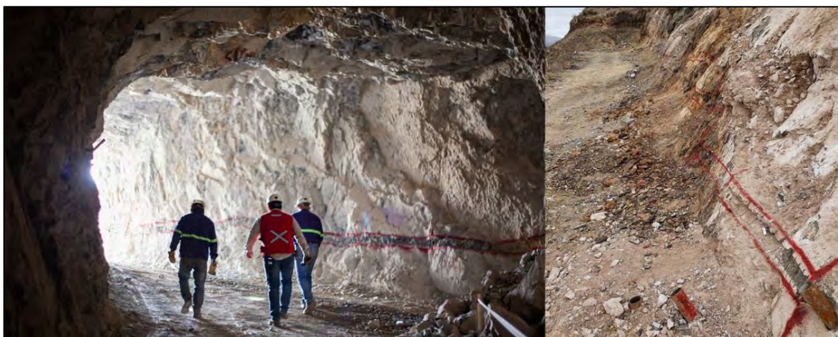
Figure 8-2: Left: channel sampling limestone in the decline at Norte completed by CMEC in 1999. Right: Channel sampling at the Limestone – siltstone contact at Muchilera..
