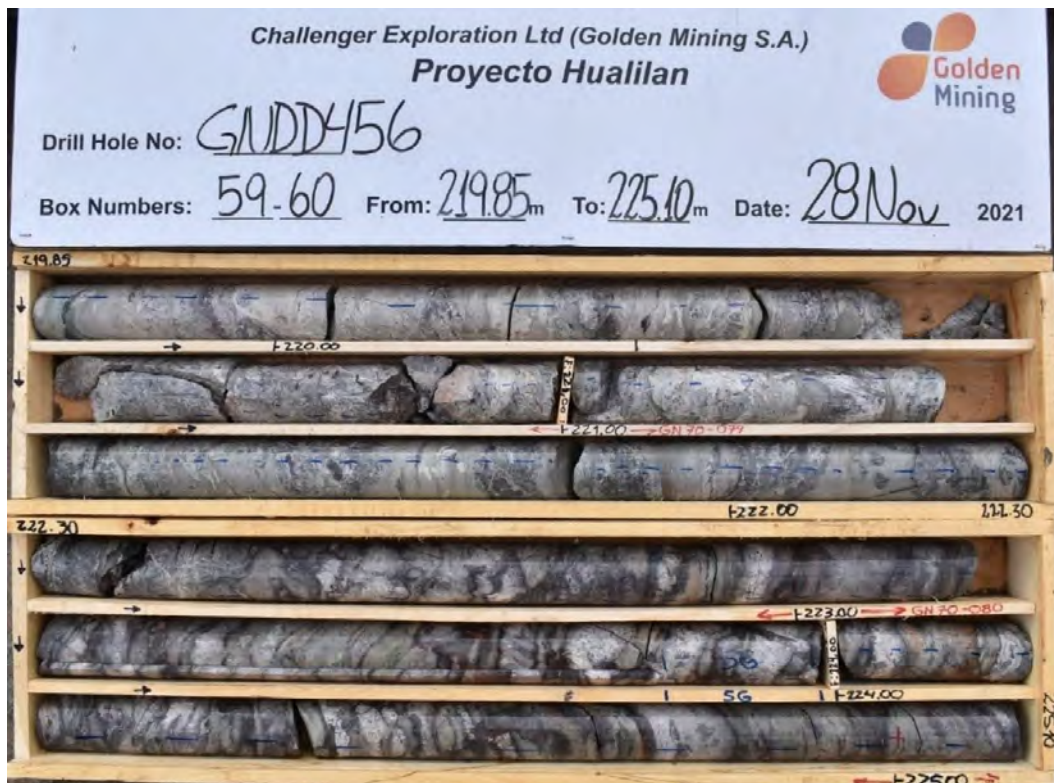
Figure 7-17: Skarn alteration in siltstone with overprinting narrow vein and disseminated mineralisation.
