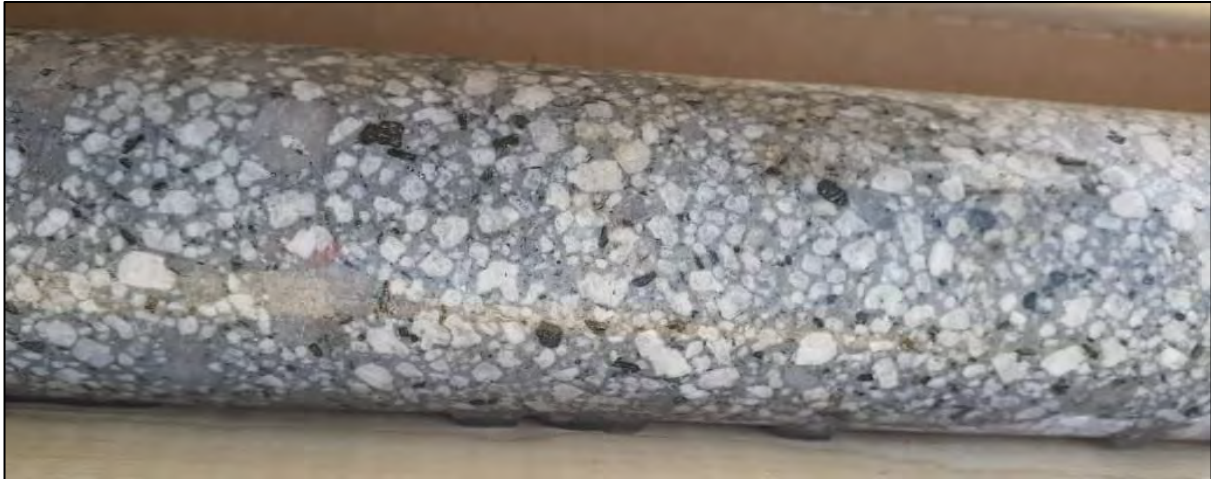
Figure 7-9: Weakly altered biotite phryic dacite porphyry in GNDD374 at 340m (Na+K is 5.8%, Al is 8.5%), drilled east of the Hualilan hills.
