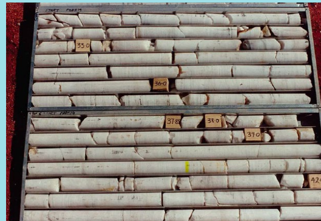
Historical drill core for hole PDDH19. Typically, pegmatitic to 28.4m then Quartz to 49.4m
