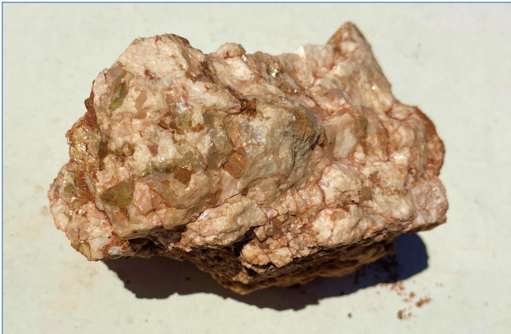
Figure 1: Fractionated pegmatite from Carr Boyd East containing Albite (70%) + Quartz (25%) + Rb Muscovite (5%) and Zinnwaldite (trace %). 2
