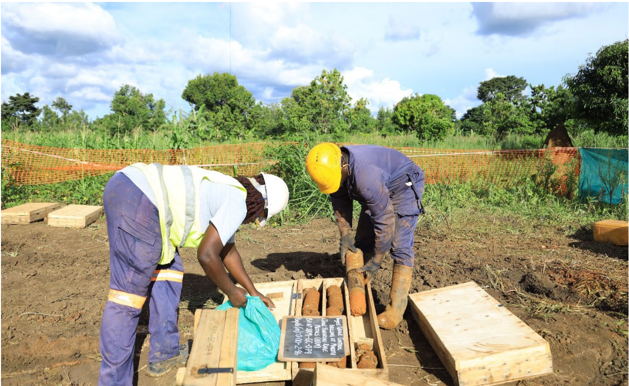
Figure 13: Grade control drilling core collection at Makuutu Demonstration test pit site No1.
