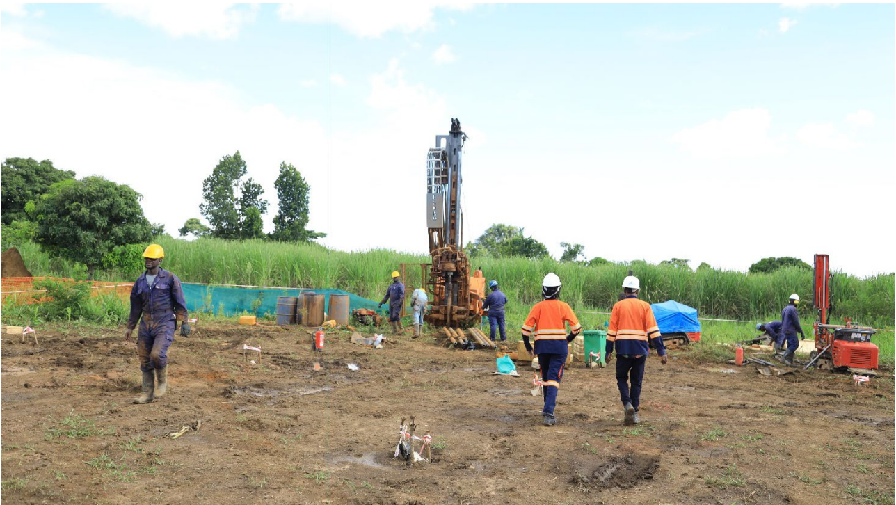
Figure 9: Makuutu Demonstration Plant test pit grade control drilling at test pit site No1 on 5m x 5m grid.
