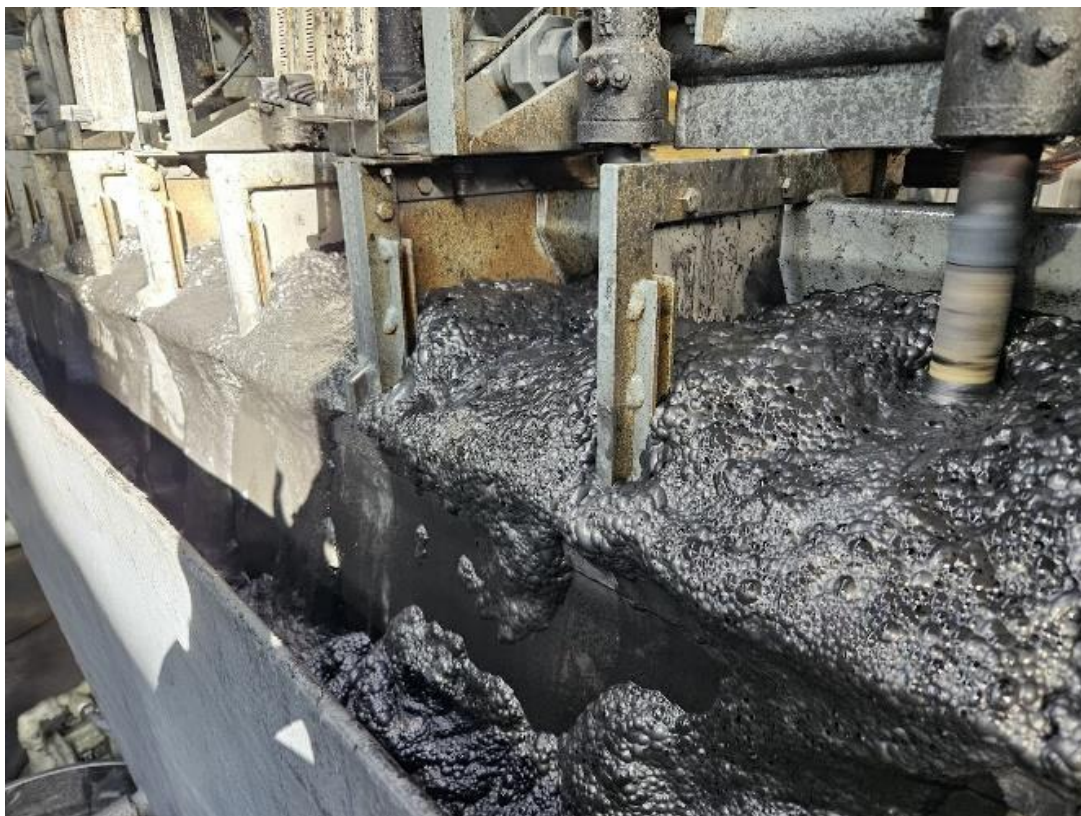
Figure 1 – Cleaner stage of bulk flotation test on Sarytogan Graphite underway at IMO in Perth, September 2023.
