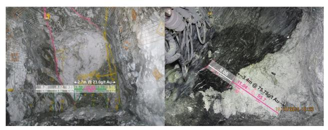
Figure 2: Photo of face 766\_400\_12 (refer Figure 5) with a composite sample of 2.7m @ 23.00g/t Au (left) and face 441\_700\_12 (refer Figure 6) with a composite sample of 3.4m @ 75.78g/t Au (right). Neither of these drives were ever stoped with mineralisation not closed off above.
