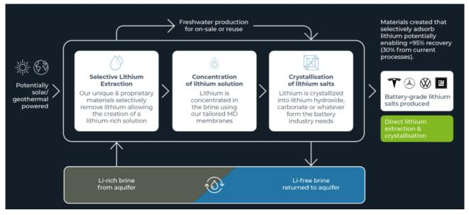
Figure 3: Watercycle's DLEC<sup>™</sup> Process overview highlighting the three stages of selective lithium extraction, brine concentration & crystallisation
