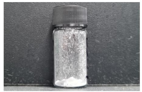
Figure 2: Lithium Carbonate directly extracted from lab-synthesised brines to match Cesano well C1
