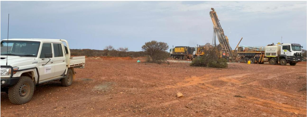
Figure 1. Orlando Drilling reverse circulation rig commencing drilling at the Southern Star prospect.
