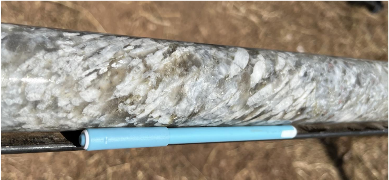
Figure 10: Spodumene mineralised core in BDFS05, mineralisation over most of intersection thickness
