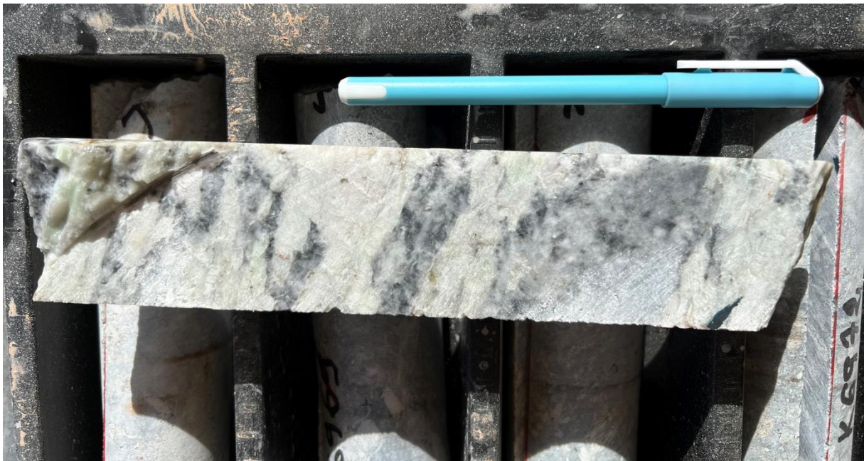
Figure 11: Large crystals of Spodumene as seen in the split core
