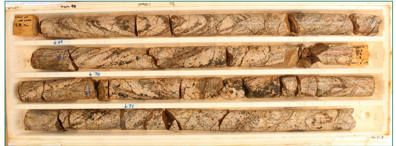
EAL007 Niobium-REE carbonatite 68-71.7m (part of 19m @ 1.0% Nb 2 O 5 from 65m)
