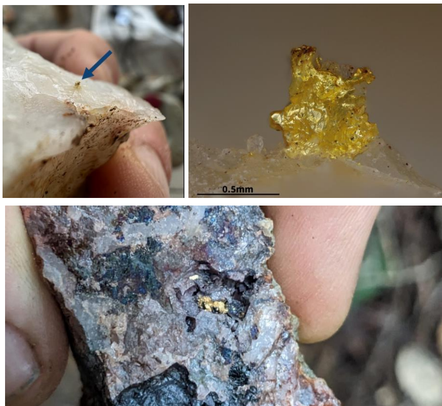
Figure 4: Visible gold in bucky quartz at the SATR001 trench (upper images – Sample R0450X) and sample R0357 (429g/t Au) from the nearby historical trenches 1
